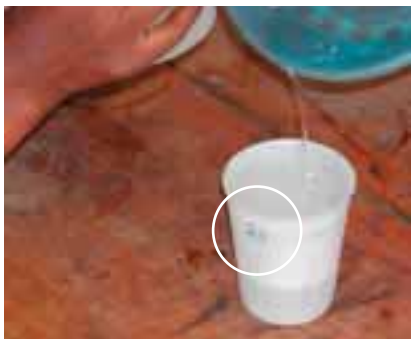
Labeling a collection cup with a black permanent text or a chinagraph pencil.
