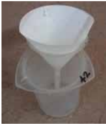
10. Fold a circular piece of filter/tissue paper into quarters, then open it as a cone and place in the funnel which is held in a beaker or stand.
