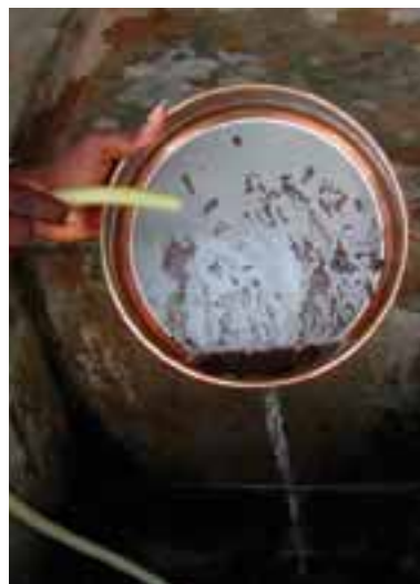
7. Rinse down each of the 2 catchment sieves, backwashing where necessary.
