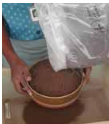
1. Coarsely sieve the sample to remove debris and lumps.
