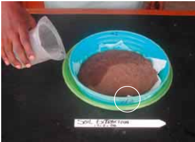
Labeling an extraction tray with both an accompanying plastic tag and also number on tray with a permanent marker or chinagraph.
