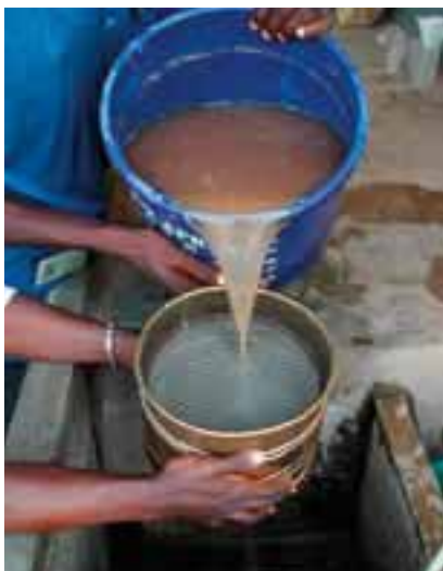
6. Slowly pour half of the water through the 2 mm, 250 and 150 \mu\text{m} sieves.
