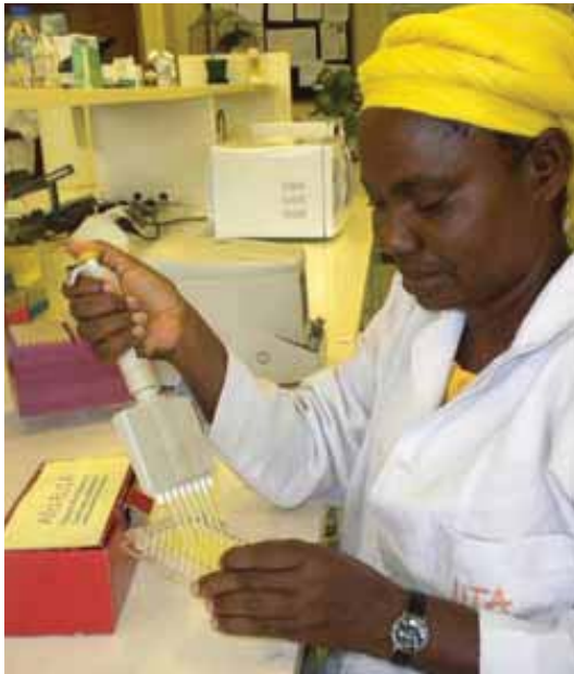
Aflatoxin testing using Afla-ELISA. Source: L. Kumar
