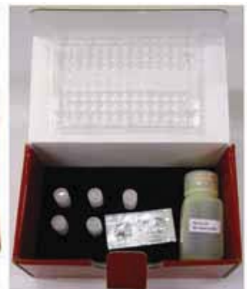
Prototype Afla-ELISA kit—a quantitative serological assay for the estimation of total aflatoxins in maize and other commodities, using 96-well microtiter plates. Up to 20 samples can be tested in each 96-well plate at a cost of US$4 per sample. Source: L Kumar.
