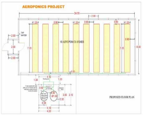
Figure 8. Schematic drawing view of AS boxes in screenhouse and the adjacent power house.
