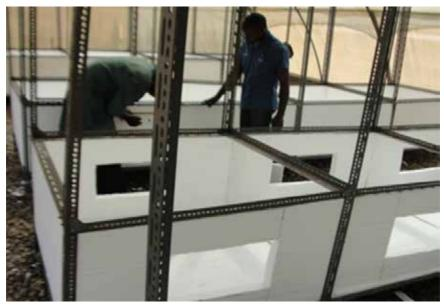
Figure 10B. Construction of the body and windows of aeroponics boxes using styrofoam.
