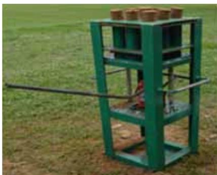
Photo 2a. A multi-piston briquetting machine developed at AfricaRice Center
