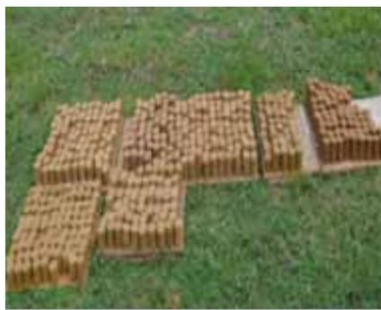
Photo 2b. Drying of briquettes at ambient conditions to moisture content of 20%.
