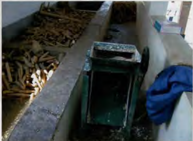
A grater which is used for starch extraction
