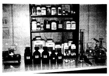
**Figure 3.** Medium preparation from stock solutions. From left to right: balance with sugar being weighed, MS mineral salt stock solutions in dark bottles, vitamin and growth regulator stock solutions in volumetric flasks, graduated cylinder with distilled water, pH stick, boiling flask.
