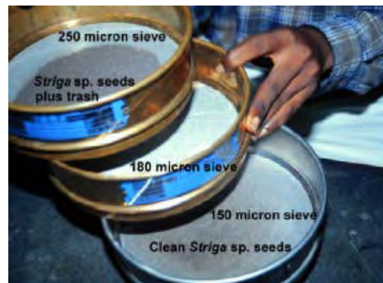
Figure 21. Freshly collected and dried Striga seeds need to be cleaned of trash by passing through a series of sieves.
