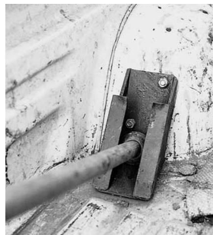
1. Forward tripod legs are pivoted near rear wheel wells.
