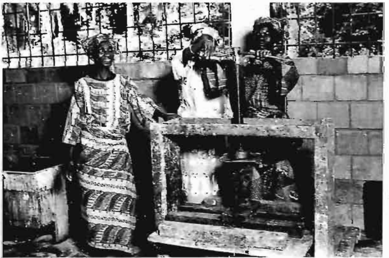
Figure 9.11 Power screw dehydrating press
