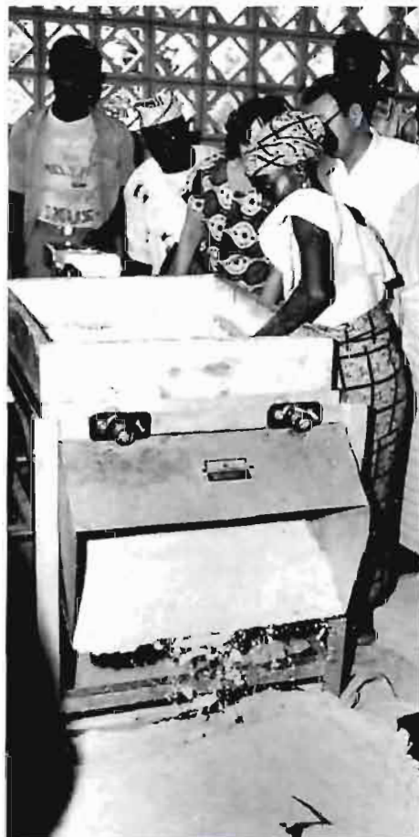
Figure 9.12 Mechanical sifter for cassava mash and gari
