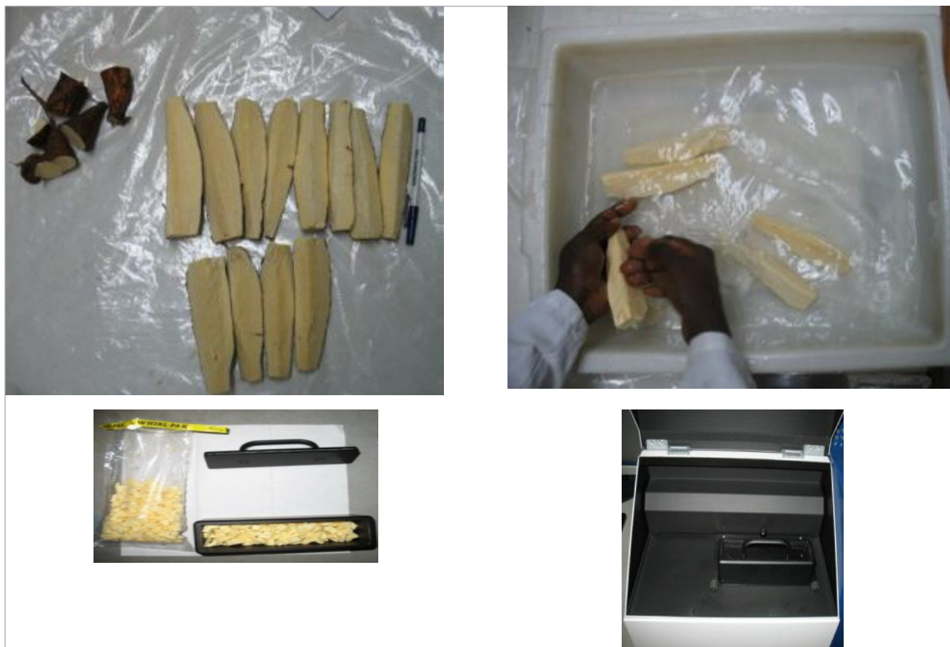
Figure 1. Sample preparation work flow of NIRS analysis in fresh cassava roots sample.
