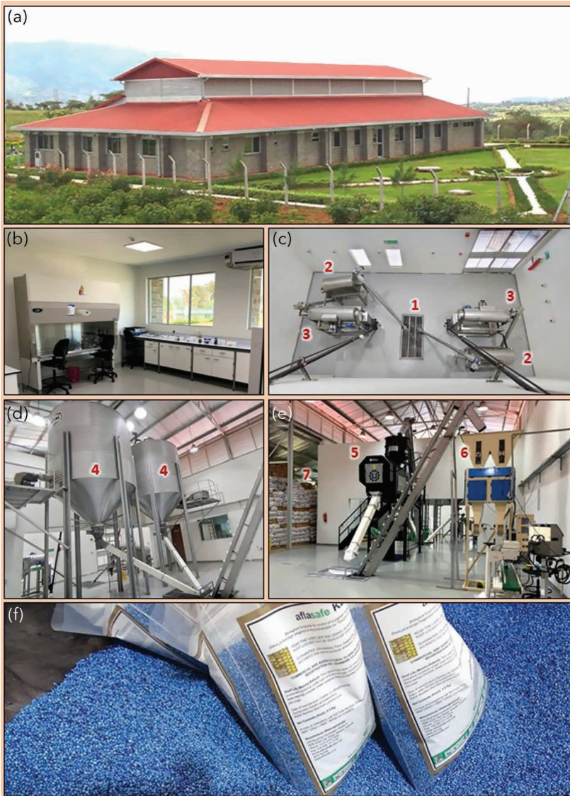
Figure 2 The KALRO/IITA Aflasafe Modular Manufacturing Plant at Kenya Agricultural and Livestock Research Organization (KALRO) Katumani Research Station in Kenya. (a). A side view of the manufacturing plant. (b). The plant consists of a laboratory where the inocula of the active ingredients are produced and combined with a blue dye and polymer sticker. (c). Carrier (sorghum) pit (1) from where sorghum is moved into a grain cleaner (2) with an auger, then transported to a roaster (3) and finally to a cooling silo for cooling and storing the roasted carrier grains. (d). From cooling silo (4), the carrier is transported via a pneumatic line into a seed treater (5) where the master solution (inoculum, dye and polymer) is coated onto the sorghum grain. (e).
