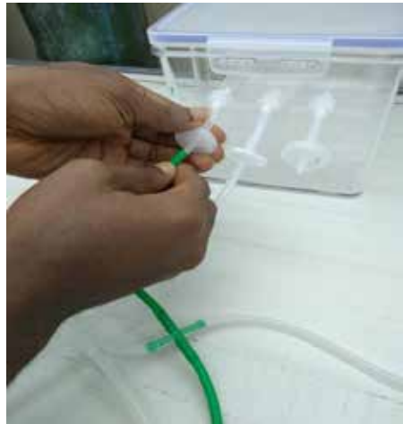
Plate 21. Setting up PF TIBS for plant introduction. Top, left: Closure of only two sides of the vessel before autoclaving; Top, right: Placement the PF TIBS into the autoclave for sterilization; Bottom right: Sterilized vessel showing “autoclaved” indicator. Bottom right: sterilized filters connected to the tubing in the flow hood
