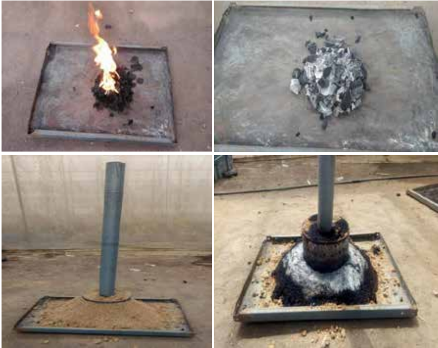
Plate 26. Making carbonized rice husk. Top row: Make a fire on a metal sheet using charcoal and allow the fire to go out but keep the glowing hot coals. Down, left: Cover with carbonizer; pour rice husk and allow to burn. Down, right: Incomplete burning will give black carbonized husk while complete burning will give whitish ash rice husk. The hotter the carbonizer, the closer to becoming ash. Both are sterile and work well for yam.
