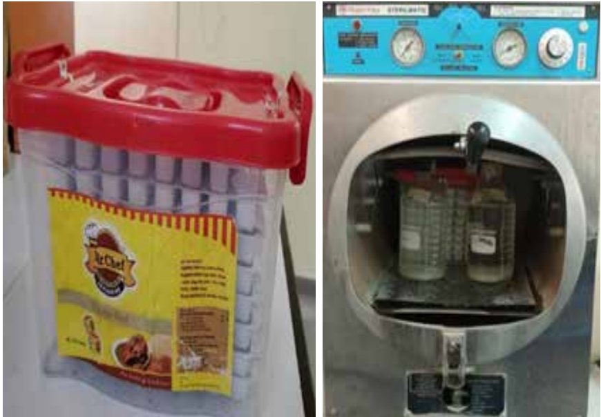
Plate 32. Stacked ViVipak trays for autoclaving (left). Two bottles are autoclaved along with the substrate (right). The first bottle contains 5.43 g of Murashige and Skoog basal medium and 1 liter of distilled water set to pH of 5.7. The second bottle contains 5.4 3g of MS + 7 g of Agar + 1 liter of distilled water, pH of 5.7.
