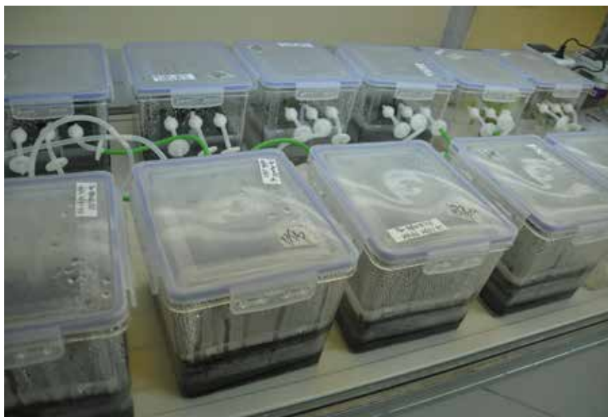
Plate 17. The Plant Form Type Temporary Immersion Bioreactor system.
