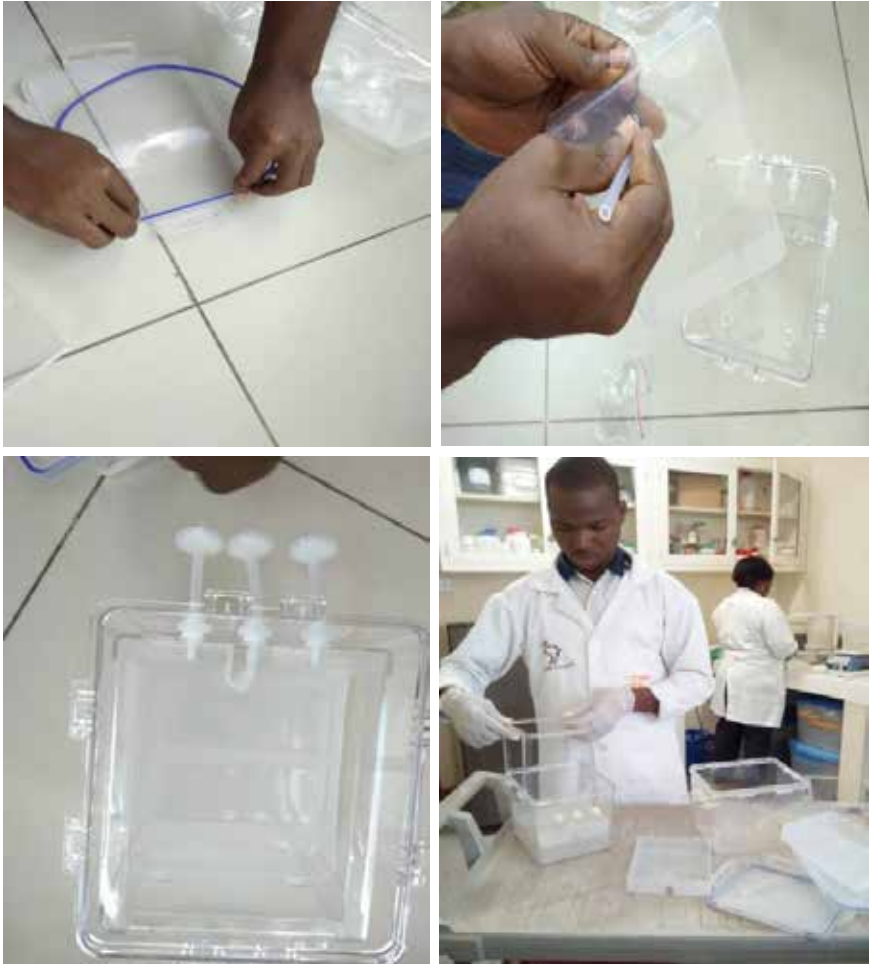
Plate 20. Connecting the parts. Inserting the silicon ring into the lid to ensure airtightness (Top Left); Silicon tube on the inner chamber to be placed on the bottom of the outer container (Top Right); Bottom left: Fixed connectors into the inlets by inserting clamp on the outer container, putting silicon ring on the clamp from the other side and screwing the nut on the clamp. Bottom Right: Inserting four-legged frame above the basket
