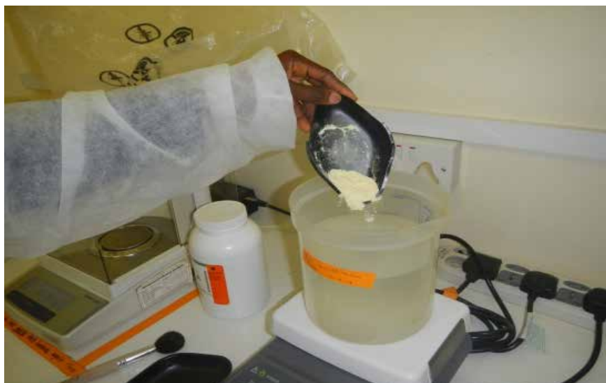
Plate 6. Preparing medium for in vitro culture of single nodes. Weighing medium constituents and pouring into distilled water in a beaker (bottom).
