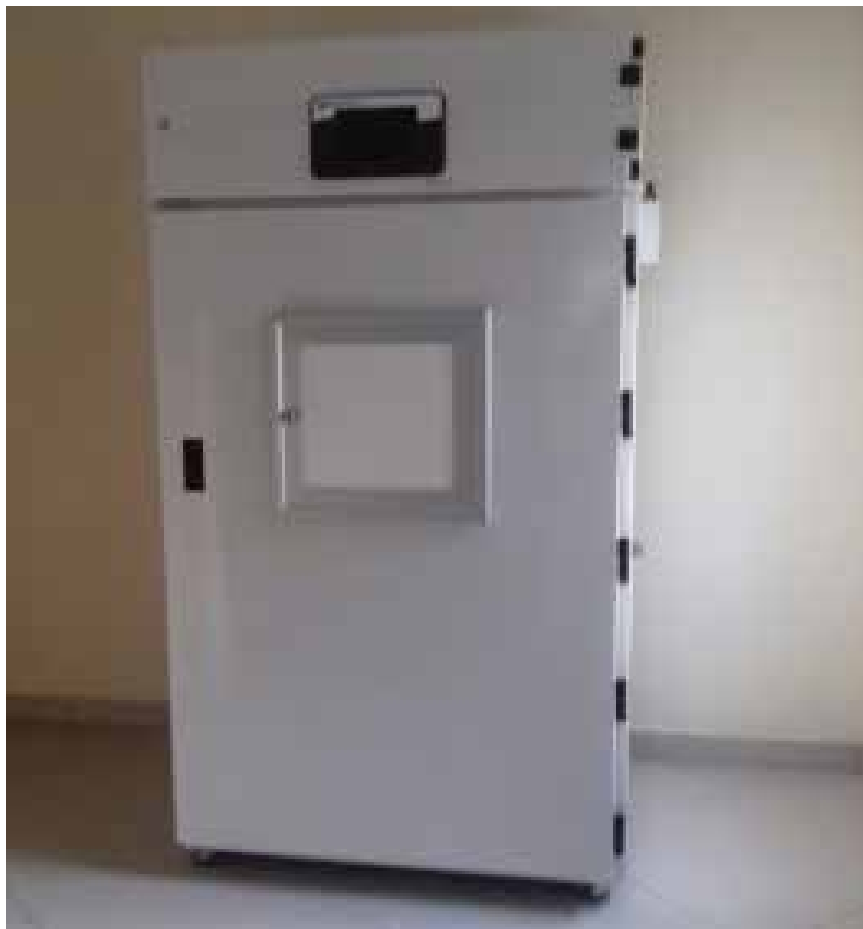
Plate 10. Temperature and humidity-controlled growth cabinet for heat treatment to clean plantlets from viruses.
