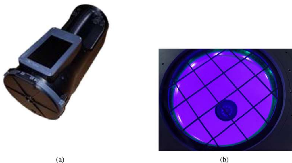
Figure 5. (a) Photo of the developed A-MSI system and (b) its LED ring and sensing chamber.
