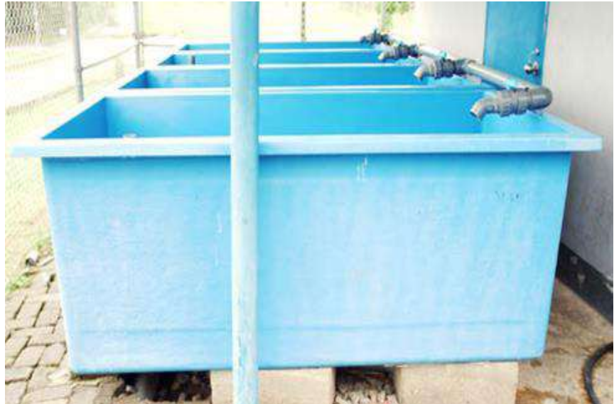
Flow-through tanks with single use of water
