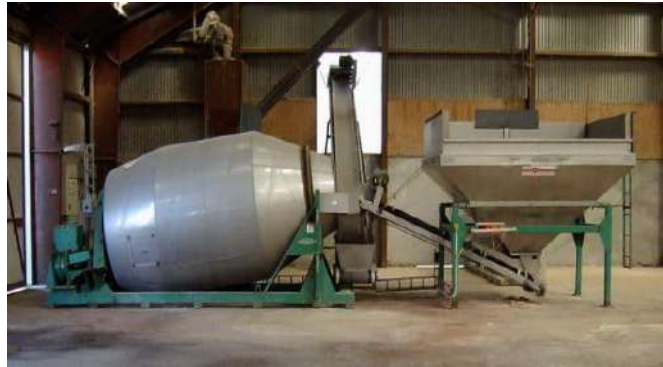
Dry rotary system used in fertilizer blending.
