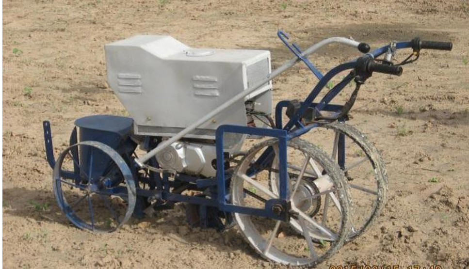
Sénékéla planter and micro-dose fertilizer applicator
