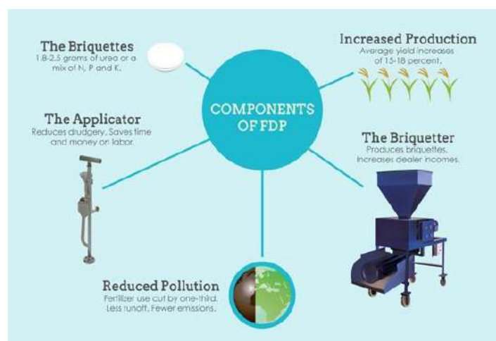
Schematic of entry points and benefits of urea deep placement technology for crops including rice.
