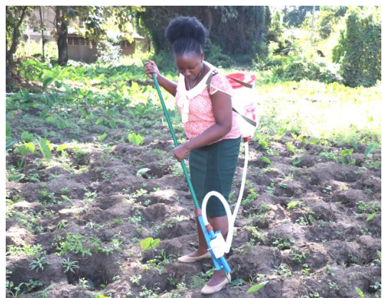
A mechanical device that delivers micro-dosed fertilizers
