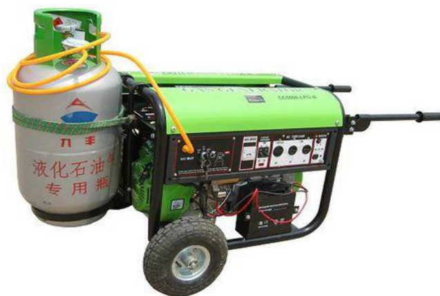
An electricity generator powered by biogas
