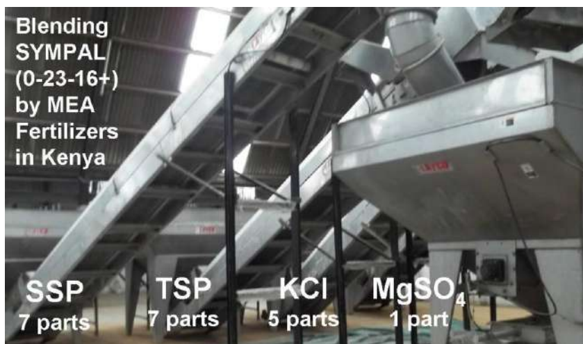
A multichannel blender in operation at MEA Fertilizers used to produce SYMPAL for grain legumes in Kenya
