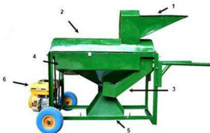
The Imara Tech Multi-crop thresher consists of a 1) feed chute, 2) threshing chamber, 3) exit chute, 4) blower, 5) seed collection chute, and 6) petrol engine
