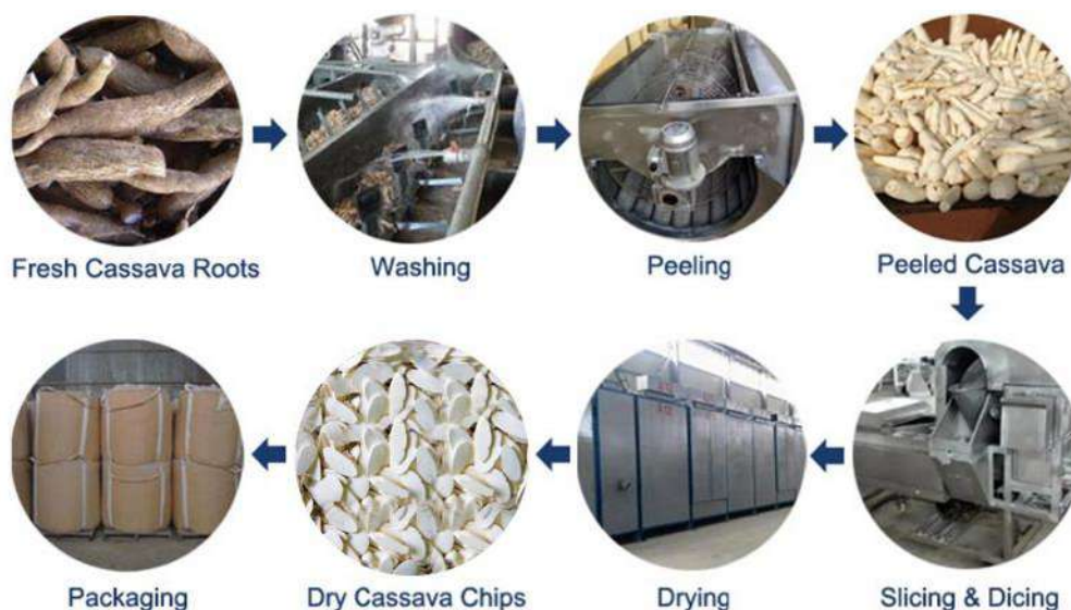
Steps of large-scale cassava chip production process.
