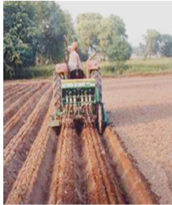
Establishing raised beds, furrows and planting rows in a single pass over a tilled and level field
