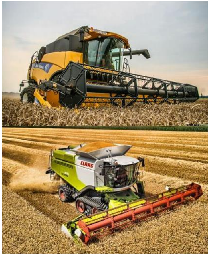
New Holland CX 8080 with 3.7 m cutting width (above) and CLAAS Lexion Combine 670 with a 12 m cutting width (below)
