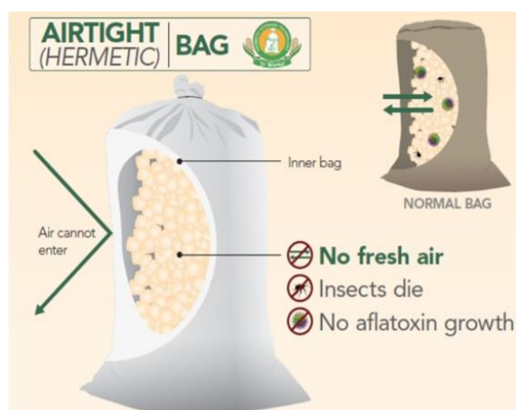
Design of a hermetic storage bag
