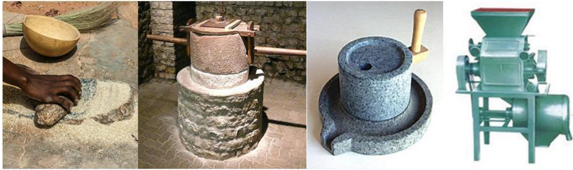
Evolution of local flour milling: traditional African grindstone (left), ancient Roman stone mill (center left), modern home stone mill (center right), small-scale electric mill (right)
