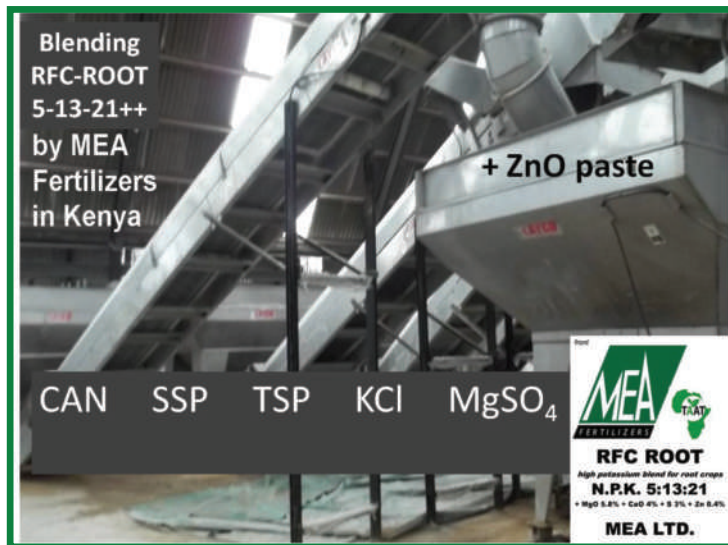
Figure 7. Blending the RFC-ROOT fertilizer by MEA Ltd. In Nakuru, Kenya (inset: fertilizer bag design).
